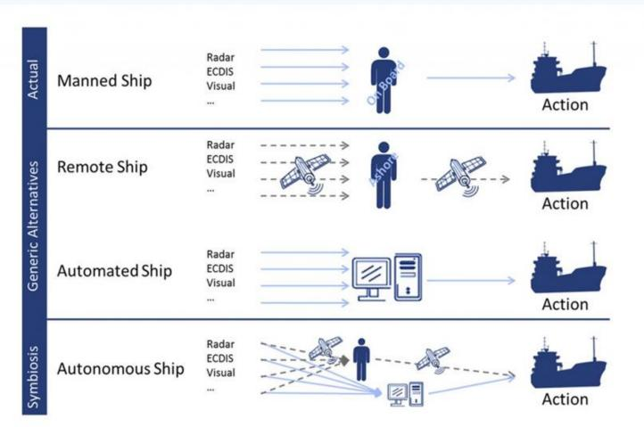
(© MUNIN <a href="http://www.unmanned-ship.org/munin/about/the-autonomus-ship/">http://www.unmanned-ship.org/munin/about/the-autonomus-ship/</a>)
