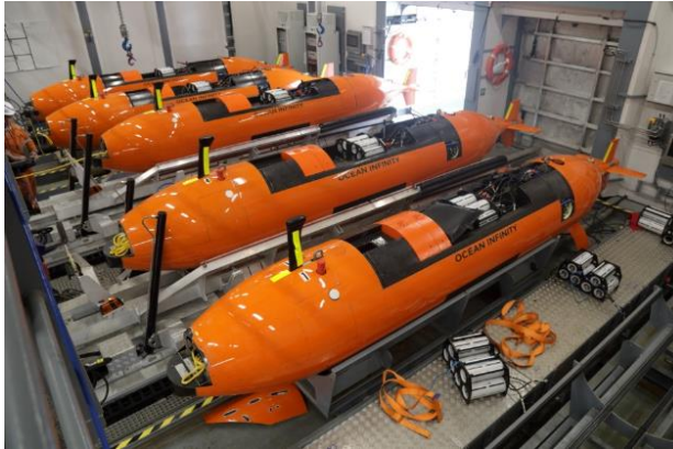
Fig. 12. Ocean Infinity's 'mothership' and deployable autonomous underwater vehicles – providing the host platform with organic assets, integrated with Launch & Recovery Systems for multiple worldwide missions [10]
