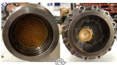
Figure 9 –Connectors continue to become denser
