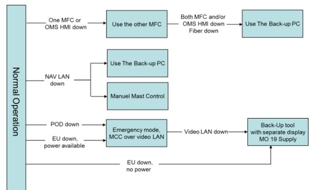
Figure 6; Overview OMS Redundancy
