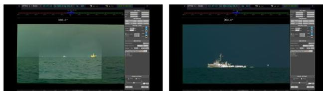
Figure 4: Image Fusion WFOV & NFOV TV/IR (50%)
