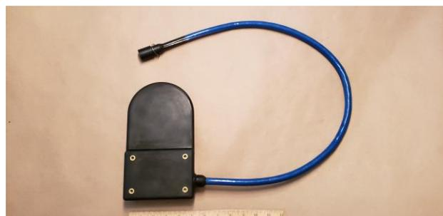
**Fig. 9.** Epoxy potted blade sensor with planar array, electronics section at the base of the sensor, and 13-wire SubConn power and Ethernet cable which powers the sensor and provides Gb Ethernet communications between the sensor and the platform. The blade sensor is bracket mounted using four M6 bolts.
