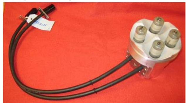
**Fig. 2.** An A-size receive array built by USSI using Calibrated Omni sensors for mammal detection using the Liquid Robotics WaveGlider towfish.
