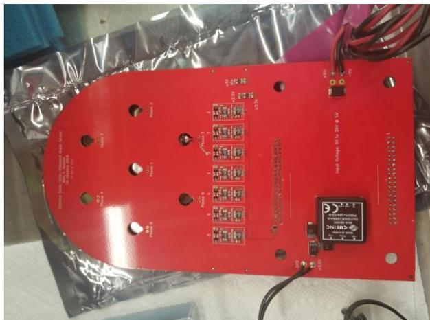
**Fig. 6.** Pre-potted blade sensor with seven ½cm phones in a hexagonal configuration. Preamp-digitizer electronics, power supply and COTS FPGA board are mounted on the same PCB.
