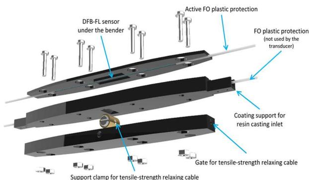
Fig. 1. SASSO sensor manufacturing
