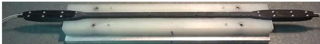
*Demolding phase after 48h curing @ room temperature*
