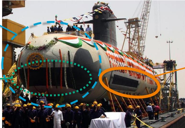
Thin planar flush mounted flank array with great surface
