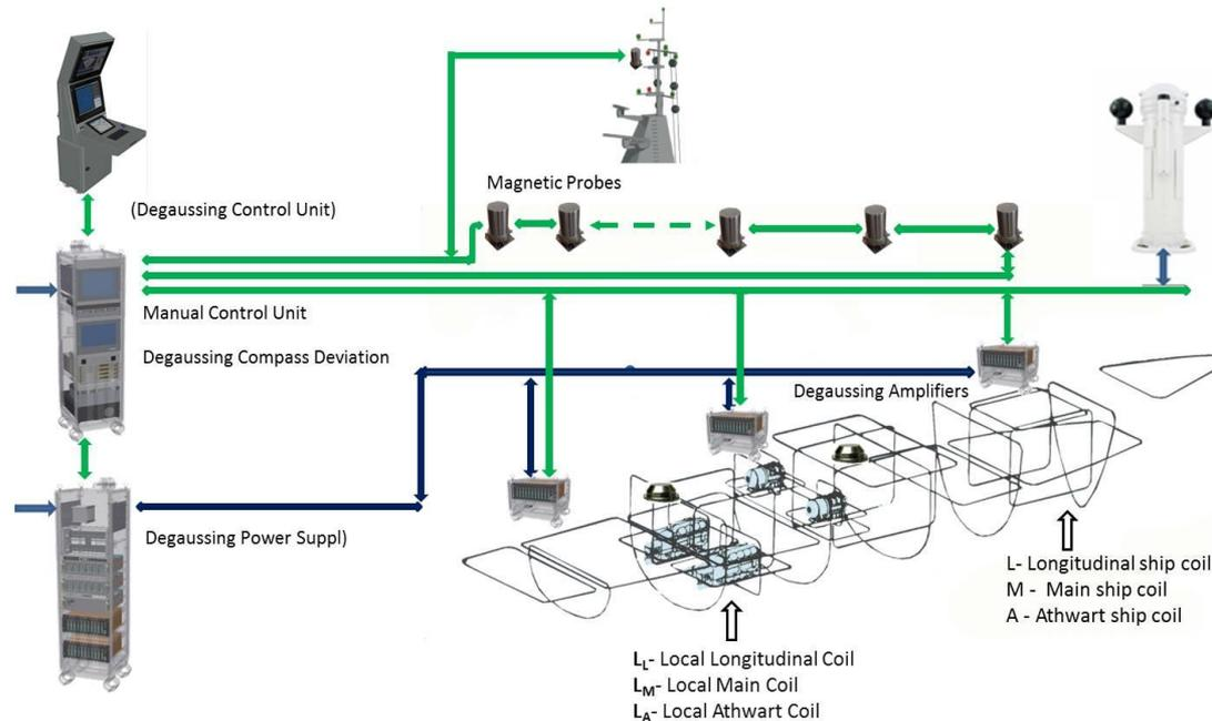
Works toward closed loop degaussing system on board new MCM vessels
