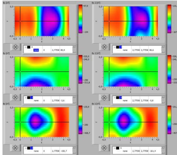
Comparison of measured (left) and recalculated (right) signature
