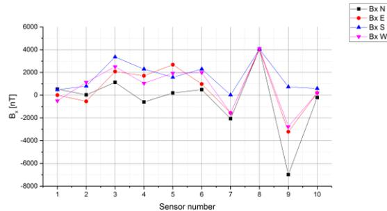
Longitudinal, athwartship and vertical magnetic field components change with course measured by sensors on board
