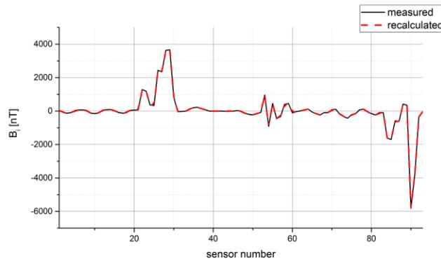
Comparison of measured and recalculated raw signature
