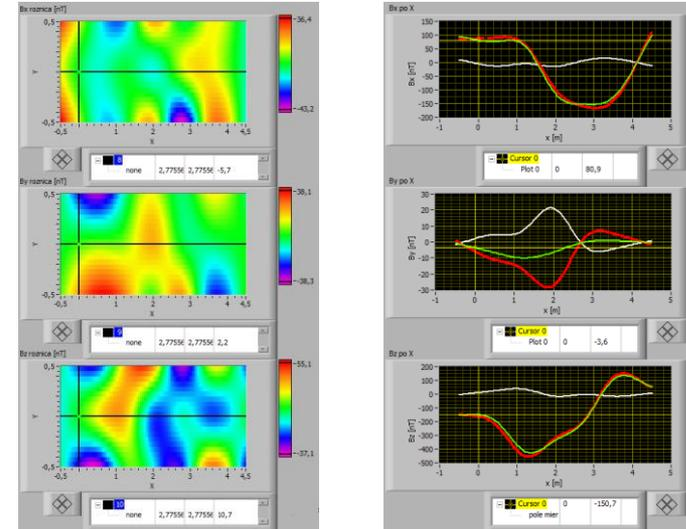
Recalculation error on surface under PSM (left) and under the keel (right)
