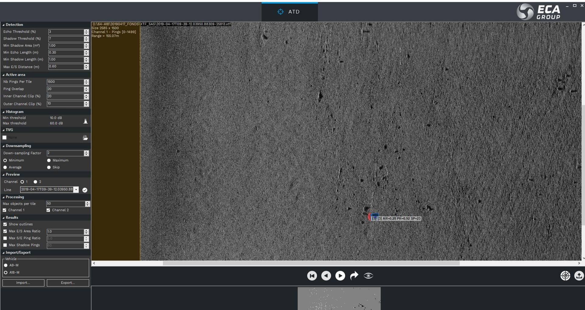
The screenshot displays the ECA ATD software interface. The main window shows a sonar scan with a detected object highlighted in red and blue. The object is labeled with the text: [9] [3] AR=0.28 PR=0.92 SP=23. The interface includes a left sidebar with various settings and a bottom control bar with navigation icons.
