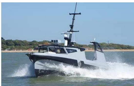
Figure 1 Unmanned Surface Vessel
