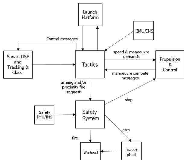
Figure 1: Simplified Torpedo Block Diagram Showing Where Tactics Sits With Respect To Other Parts of the System
