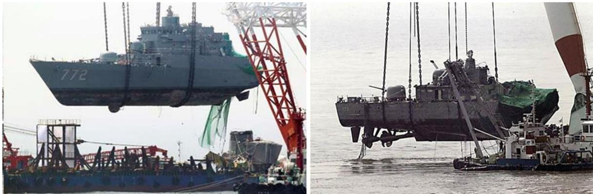
**Fig. 1.** The ROK Navy Cheonan was torpedoed in 2010. After the torpedo impact it broke into two main parts and sank rapidly.
