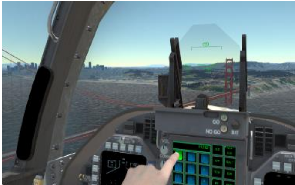
Figure 7: Green highlight provided when the finger is contacting a button.
