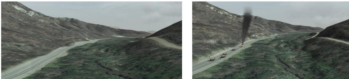
Figure 2: A comparison of rendered 10m elevation (left) to 1m elevation (right), draped with the same 1ft imagery as displayed in VR-Vantage.
