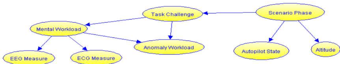
Figure 6: A possible model for the estimation of the Mental Workload of the trainee, including sensor model, context and anomaly pattern.
