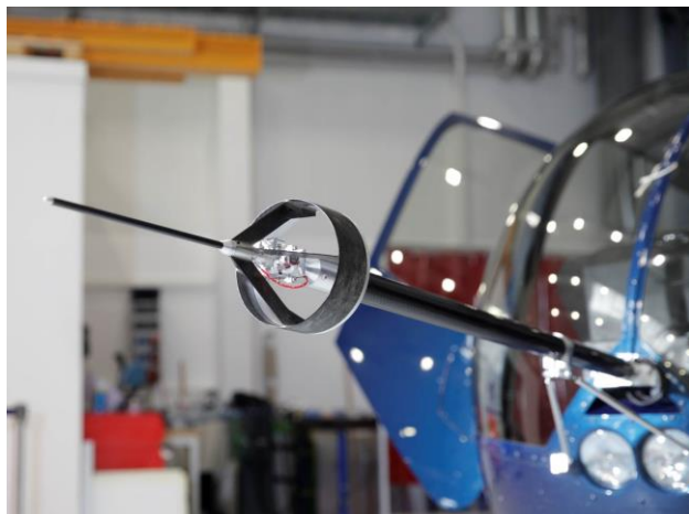
Fig. 3 AFLS mounted on nose boom
