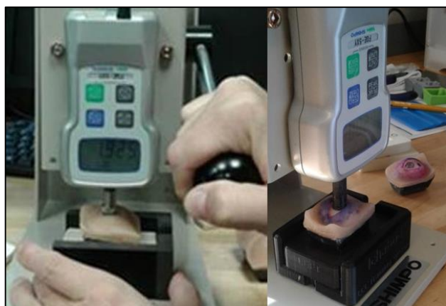
Fig 3. The empirical testing apparatus that was used during evaluation of the LCC training system [4].
