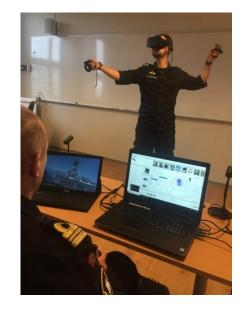
1 x 17" Laptop with NVIDIA Quadro P4000: 1 x Universal Serial Bus (USB) portable screen 1 x Oculus VR HMD + VR Controllers 1 x Microsoft Kinect Sensor 1 x Xbox 360 Gaming Controller 1 x Pelicase
