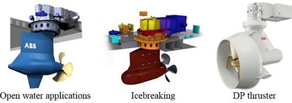
Fig. 2. Examples of different marine electric propulsion systems [5].
