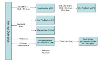
Figure 6; Overview OMS Redundancy
