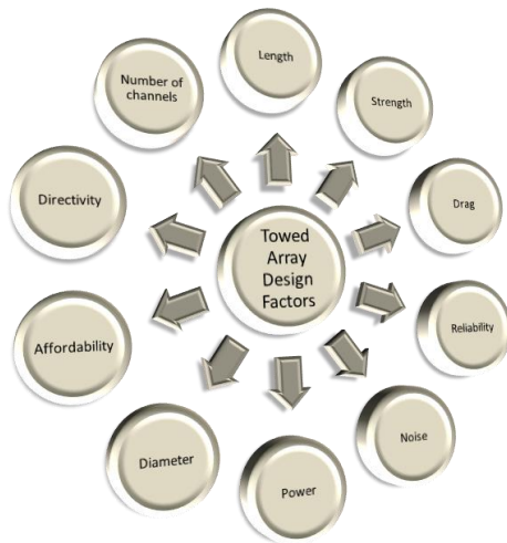
Figure 1 - Key design factors for towed arrays
