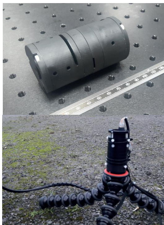
Figure 7 – MagCell Magnetometer on Optical Bench (top) and On Tripod at Underwood Quarry (bottom)
