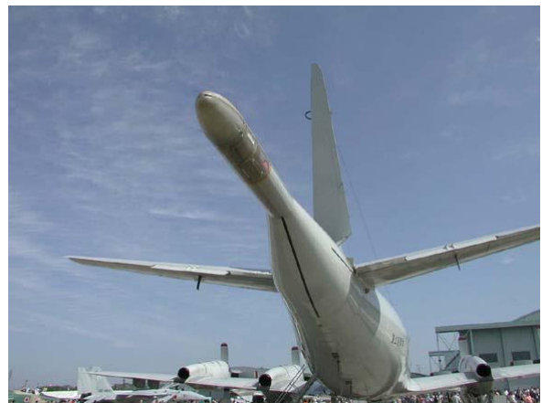
Figure 2 – MAD Rear Boom Mounted on Orion P3-C Aircraft
