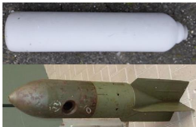
Figure 9 – Ferrous Gas Cylinder (Static Magnetic Target) and SC-50 Aerial Bomb
