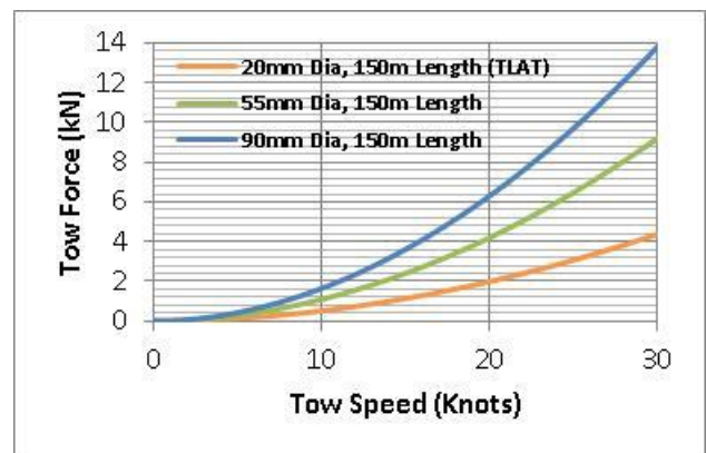
Fig. 4. Indicative Towed Array Hydrodynamic Drag
