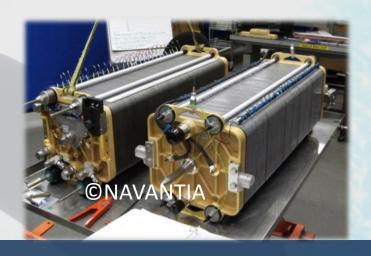
Specifically developed to military naval specifications. Not a commercial based PEM adapted to submarine use.
