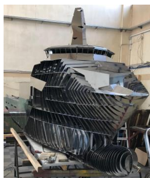
Fig. 9. Ferromagnetic PSM under construction
