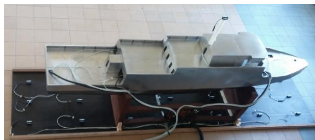
Fig. 3. PSM with test stand and sensors on board
