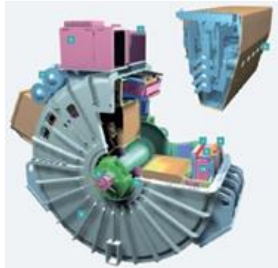
Main Propulsion Motor
