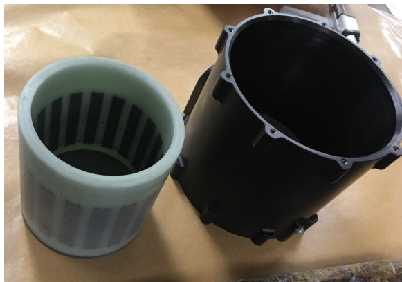
Figure 12. Sealing pole piece array before insertion into gear casing.
