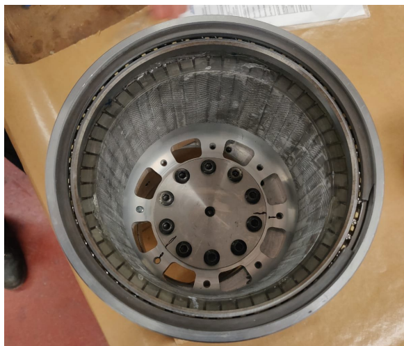
Figure 13. Magnetic gear final drive rotor
