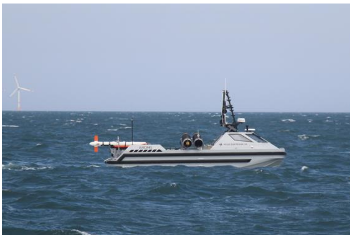
Figure 1. ARCIMS USV as part of the UK Sweep Capability (top) and with the AQS-24B towed SAS and Seafox mine disposal system (bottom). The USV can also launch and recover the SeaCat UUV.
