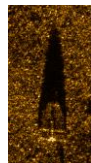
Figure 10 High Resolution imaging of a wedge target on an easy environment. Approximately 1*1 inch resolution. Note that the point of view of the object is here relevant for classification. It may not be the case all the time when objects can be deployed at any orientation over 360 degrees. There are some object significant points of view that operators should not miss to obtain good classification performances.
