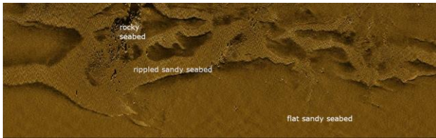
Figure 3: Different environments on a sonar image.
