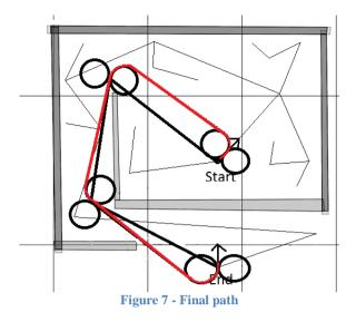
The waypoints in the final path are then drip-fed, one by one, in the behaviour based layer and the waypoint behaviour is responsible for achieving each waypoint in turn. The actual path taken by the USV may be seen in Figure 8.
