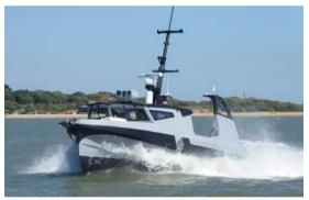
**Figure 1 Unmanned Surface Vessel**
