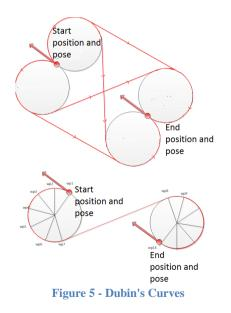
After the initial RRT tree is computed it is searched for the shortest path from the start to end position. The shortest path is then processed to optimise its geometry. Nodes that are in direct line of sight of each other are directly connected cutting out any intermediate nodes and
