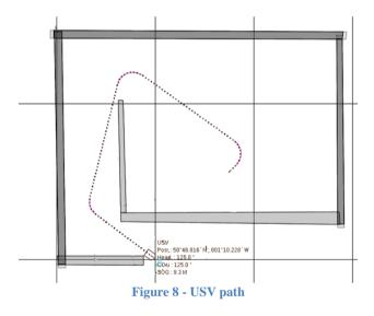
It should be noted that the behaviour based autonomy on its own would never find its way past this simple configuration of objects to find a way to the end point, but would become stuck on the "starting side" of the objects.
