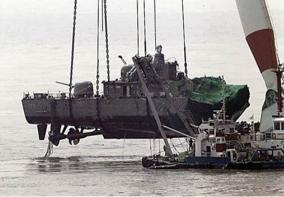
Fig. 1. The ROK Navy Cheonan was torpedoed in 2010. After the torpedo impact it broke into two main parts and sank rapidly.
