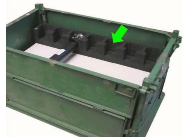
Separators for Big and/or Heavy Components & CKD Returnable Packaging
