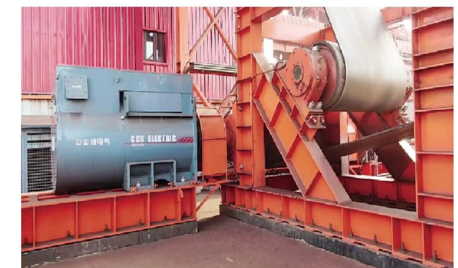
● Iron Ore Belt Conveyor 560kW/10kV Integrated VFD Direct-drive PM Motor
