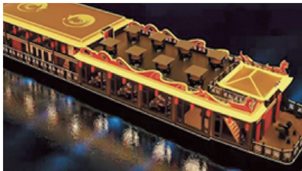
Client : Hunan Haiquan Yacht Co., Ltd. Project: 1400 kWh Tourist Boat Length: 50.8 m Propulsion Power: 225 kW * 2 Location: Guangyuan City, Sichuan Province Delivery Time: 2023
