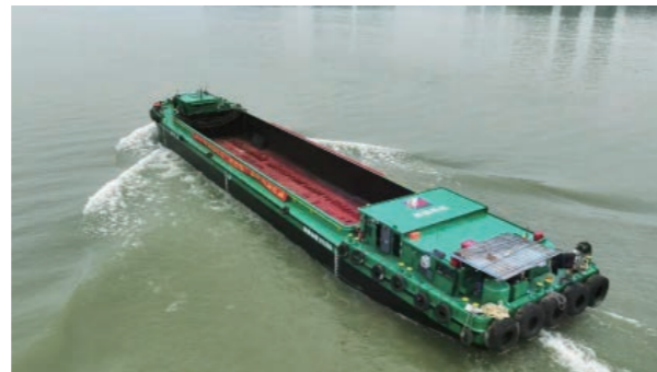
Client : Zhejiang Zheneng Mailin Environmental Technology Co., Ltd. Project: Zhejiang's First "Oil-to-Electric" Inland Freight Vessel Length: 44.8 m Propulsion Power: 200 kW * 2 Battery Capacity: 1048 kWh Delivery Time: 2024
