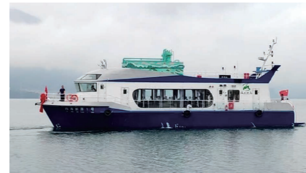
Client : Lushan West Lake Scenic Area, Jiangxi Province Project: Jiangxi's First Hydrogen-Electric Hybrid High-End Official Vessel Length: 23.65 m Propulsion Power: 160 kW * 2 Battery Capacity: 552 kWh Delivery Time: 2024
