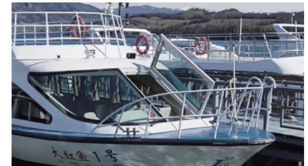
Client : Hunan Sunbird Holding Co., Ltd. Project: 630 kWh Tourist Boat Length: 28 m Propulsion Power: 55 kW * 2 Location: Jinhai, Beijing Delivery Time: 2021
