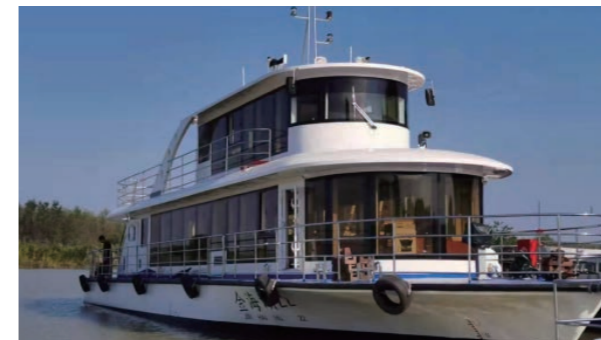
Client : Changzhou Donghai Yacht Co., Ltd. Project: 560 kWh Tourist Boat Length: 20.8 m Propulsion Power: 45 kW * 2 Location: Kanas Lake, Xinjiang Delivery Time: 2021
