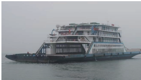
Client : Chuanjiang Roll-on/Roll-off Ship Company Project: Chuanjiang 130m Type II New Energy RoRo Ship Length: 130 m Propulsion Power: 550 kW*6 + 500 kW side thruster Battery Capacity: 1989.12 kWh * 2 Delivery Time: 2025-2027
