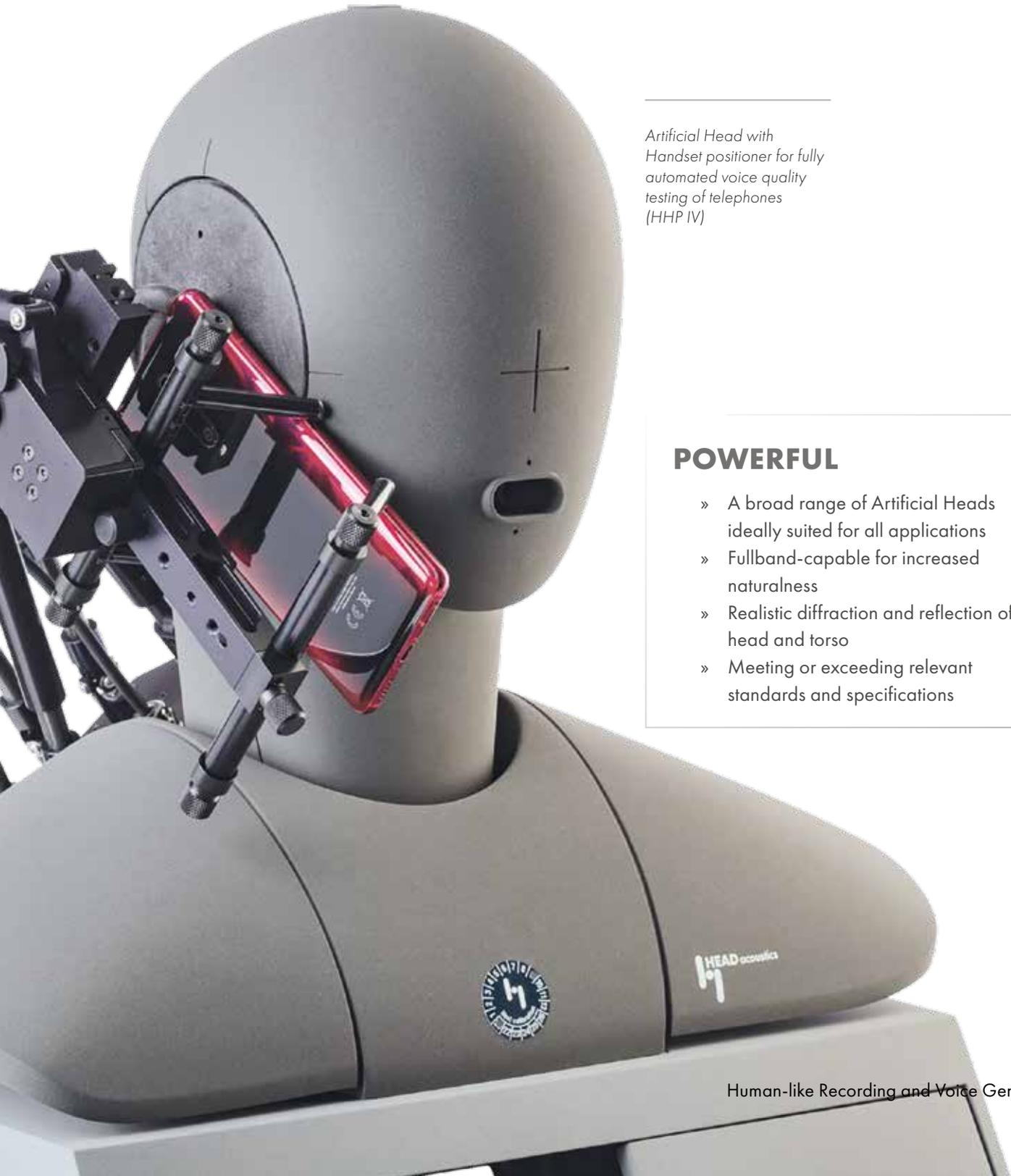
*Artificial Head with Handset positioner for fully automated voice quality testing of telephones (HHP IV)*
