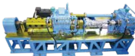
Spinning Torsion Tester with Power Recycling System
