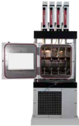
Creep testing machine with up 5 axes
