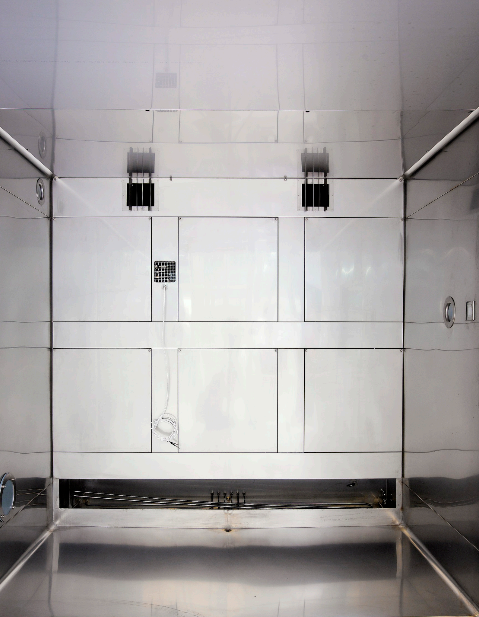
WALK-IN ENVIRONMENTAL TEST CHAMBER
