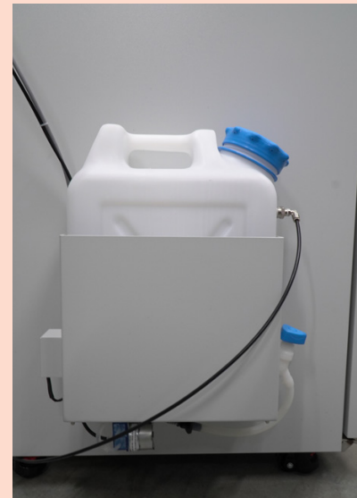
Water supply tank
