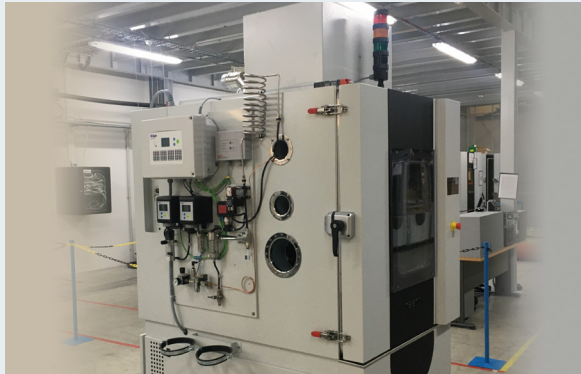
TESTA BATTERY TESTING CHAMBER
