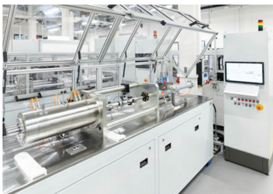
The system inspects rod seals with diameters ranging from 17 mm to 70 mm for wear, leakage, and friction.
