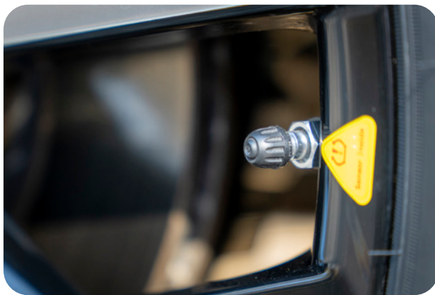
Figure 6 - Hardware TPMS sensor mounted on COMPREDICTOR
