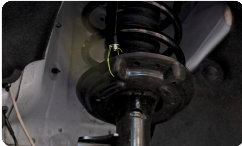
Figure 7 - Suspension Displacement hardware sensors mounted on COMPREDICTOR
