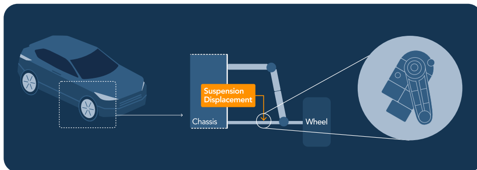
Figure 2 - Illustration of hardware Suspension Displacement sensor
