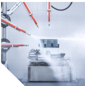
ingress protection testing - IP9K
