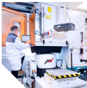
vibration testing with temperature superposition
