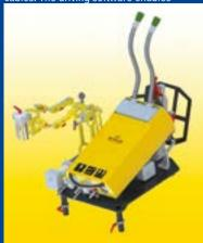
repeated operation with different driving styles. Its performance is identical to that of SAP2000 on a chassis dynamometer, which ensures best traceability in the development and verification of vehicles.
