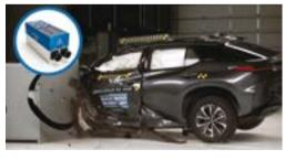
system records measurements during dynamic testing. The DTS FMVSS305 features a standard 19-pin comm interface that supports ethernet communication, DTS signals (start/event/status) and manual resistance test switches. It easily connects to external voltmeters and pendants, making it ideal for demanding highenergy test environments.
