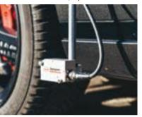
direction via an optical method based on spatial frequency analysis. It is designed to deliver unmatched accuracy, including slip angle (wheel slip angle) precision better than 0.1°, even during slow or steady driving – a critical advantage for advanced control systems, driver assistance development and autonomous vehicles.
