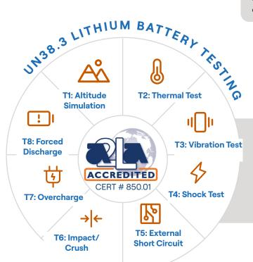
UN38.3 battery testing refers to a series of rigorous safety tests required by the United Nations for lithium batteries to ensure they can be safely transported, particularly by air. MGA's test facilities are ISO 17025 accredited for UN38.3 testing.
