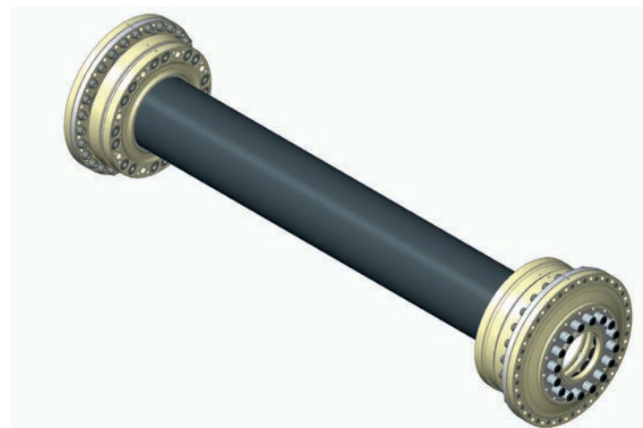
High-speed joint shaft with multi-disc clutch (up to 40.000 rpm or 2.400 Nm, 770 kW, up to 0,5° per joint)
