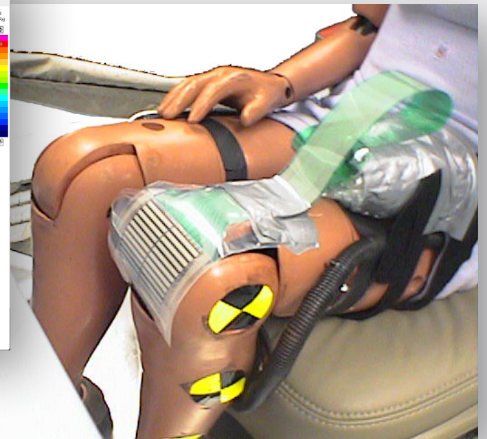
Output of Peak Pressure Exerted Upon a Crash Test Dummy's Knee During High-Speed Impact / Collision Testing
