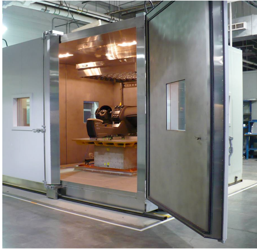
Figure 5. A Data Physics Matrix multi-DOF vibration controller runs a time waveform replication test on a Team Cube 6DOF shaker system for cockpit modules.
