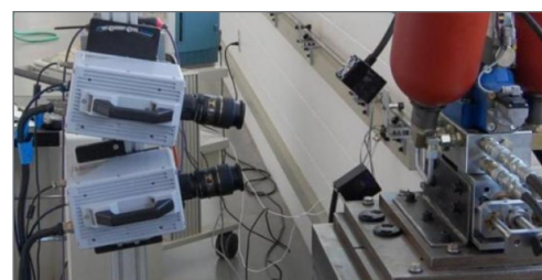
Figure 3 The VIC-3D HS system arranged vertically
